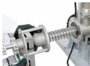
Screw-conveyor with adjustable speed
